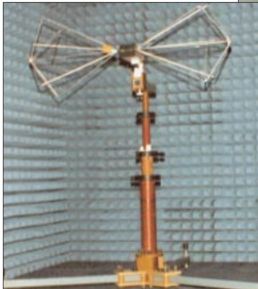
analab maintains state-of-the-art EMI/EMC testing equipment. Biconical antenna (below) and full anechoic chamber (right)
