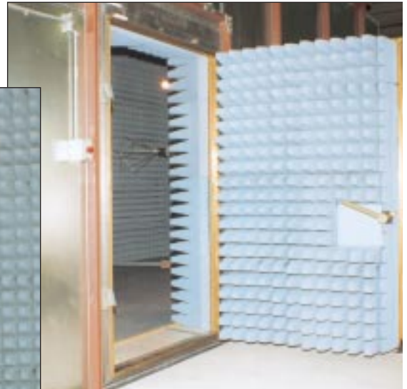
analab maintains state-of-the-art EMI/EMC testing equipment. Biconical antenna (below) and full anechoic chamber (right)
