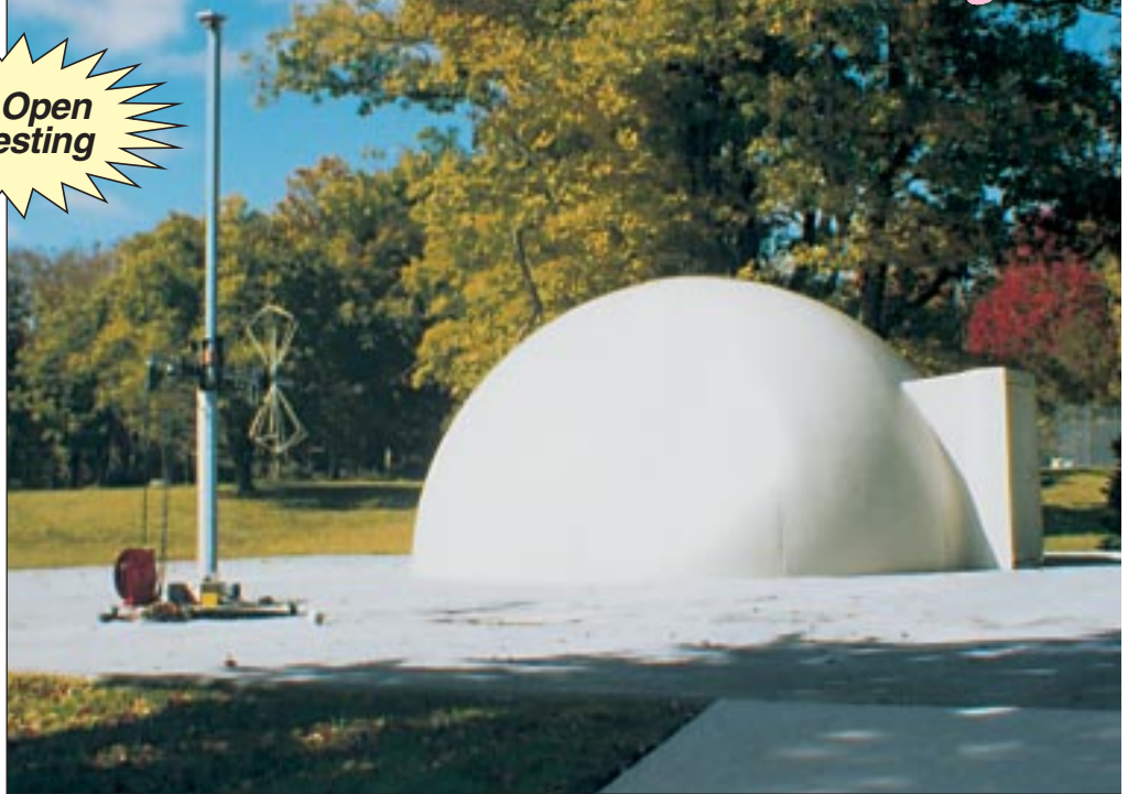
Pictured above is analab's 3 and 10 meter (OATS) Open Area Test Site used for performing emissions testing
